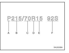
The following illustration shows an example of a typical passenger car tire size.
